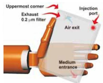
Figure 1. Shows the holding position of the Petaka™ during operations.
